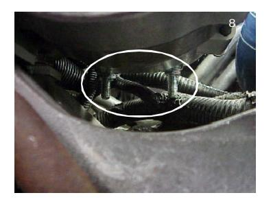
8. Rotate alternator case so that electrical posts are positioned in a downward location.
