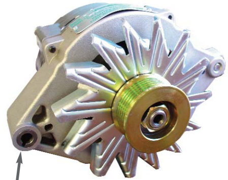
PX-2P-120 3" FOOT (PX-2P-2 HAS A 2" FOOT)
