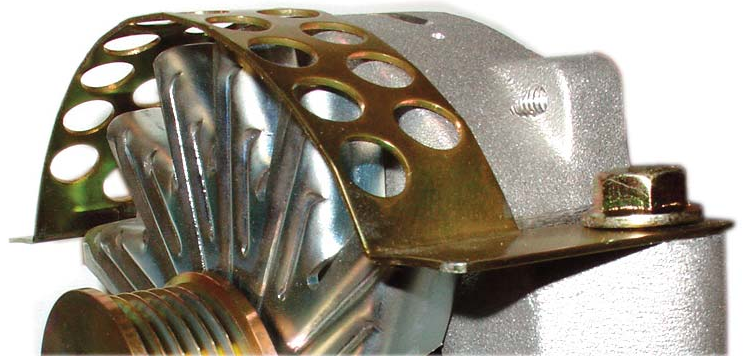
Mock-up of a fan guard installation viewed from the top.
