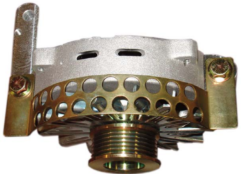
Mock-up of a fan guard installation viewed from the top.
