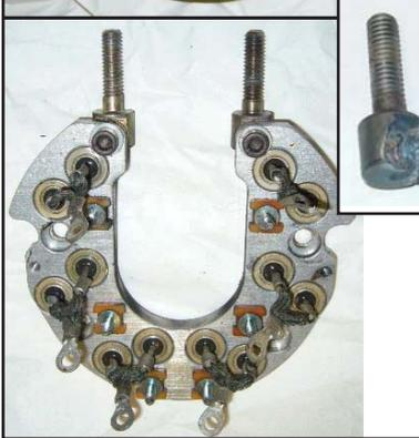
PennTex has not used the older PX-1066 style output post for almost ten years. As you can see in the inset photo on the left, the screw that attaches the post to the positive heat sink can loosen. The heat buildup from a loose connection can cause the bolt and post to weld together and the positive heat sink will be damaged. Also, please note that the old Top-hat style diodes with crimped-on braided wire leads in the heat sink are older designs that we have replaced with newer technology.
