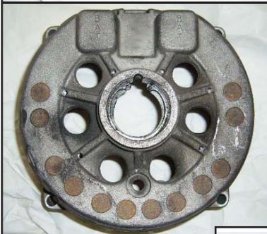
The horseshoe style flat positive heat sink that the "Non-PennTex" alternator uses is cheaper to build and quick to assemble. A heat sink like this has never been used in a Genuine PX-2 or PX-5 series alternator. The size of their heat sink actually causes airflow to be blocked as it enters through the six small holes in the rear. Die cast finned aluminum heat sinks like the ones found in Genuine PennTex PX-2 and PX-5 series alternators allow the diodes to cool more efficiently.
