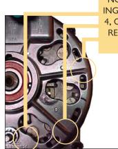
NO DIODES IN THE REAR HOUSING MEANS THESE ARE A PX-2, PX4, OR AN ALTERNATOR SOMEONE
