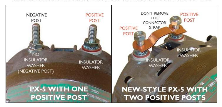
**QUESTION**: this new PX-5 alternator has a connector strap between the two big posts on the top where the cables connect. The PX-5 alternator that I took off doesn't have that strap. **Do I have to connect the Positive** & Negative cables up differently on this new PX-5 alternator?
